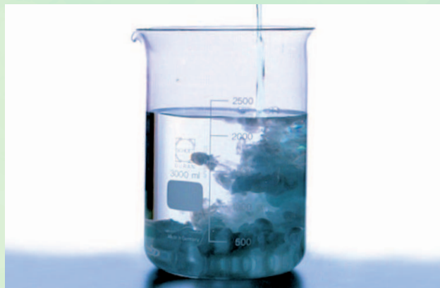
Oil with 10% IMWITOR® liteMULS poured into water
